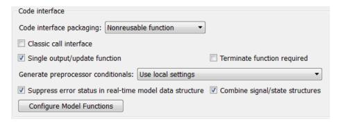
For roll, the interface settings direct the code generator to create two entry point functions to initialize and step through algorithm code.
