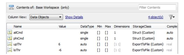
From the Simulink Editor, press **Ctrl+B** to generate code. In the code generation report, select threshold.h. In the file, find the data declarations for upThr and loThr.
